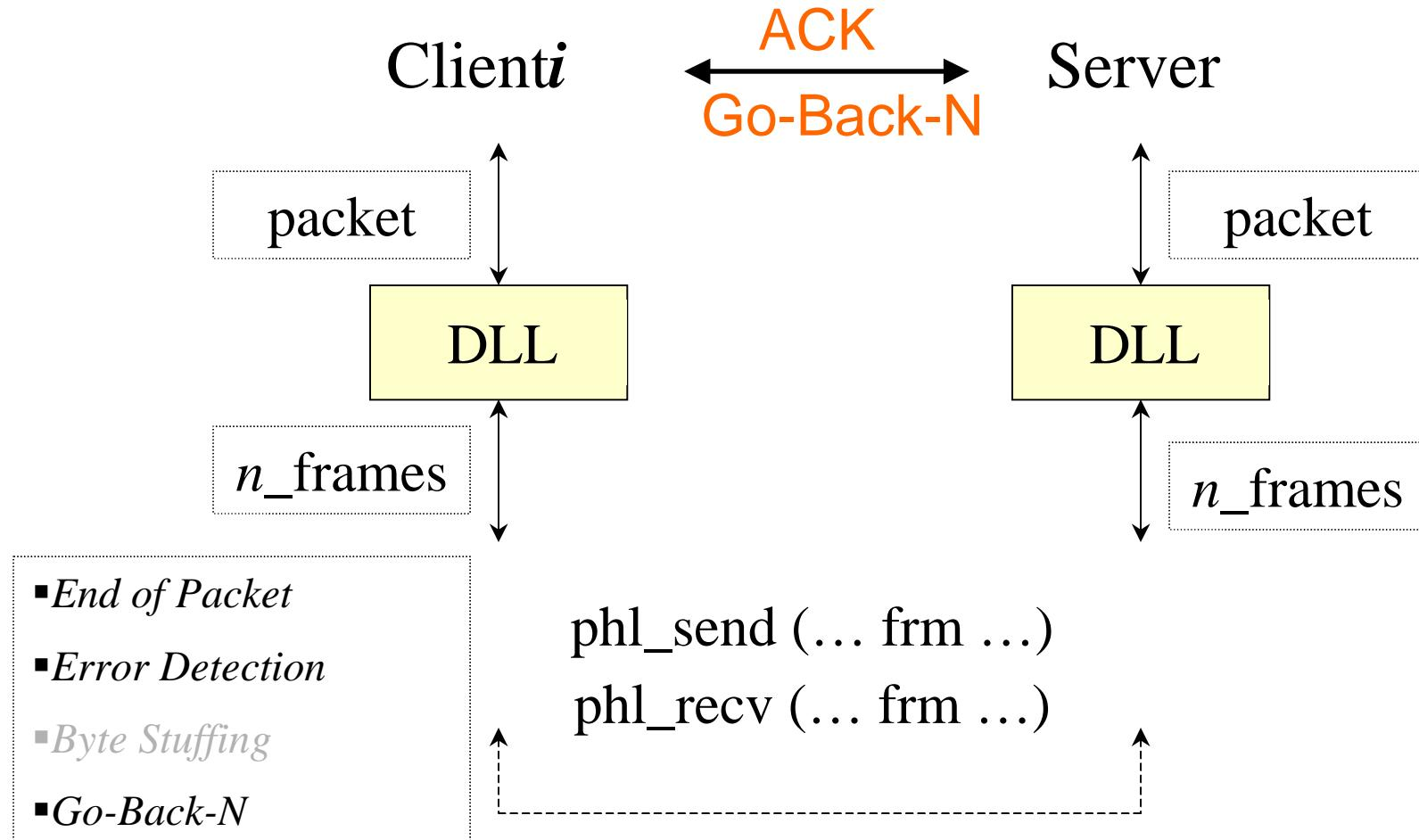
*Note: The max\_size of a frame payload is 48 bytes*
