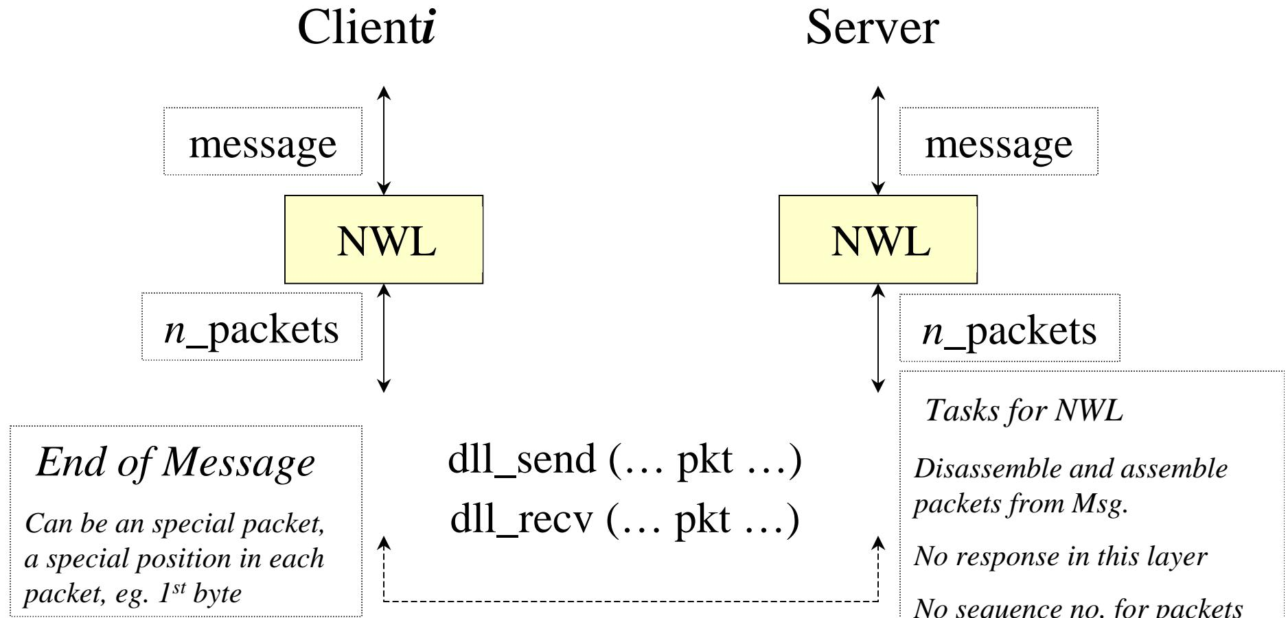
*Note: The max\_size of a packet is 72 bytes*
